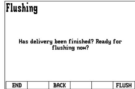
The flushing itself shows a screen, which is very similar to the delivery screen. Only the key page differs, and the flushing progress indicator in the right bottom corner is new ("F=0%").
